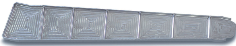
图10 采用深冷加工技术制造的大型钛合金飞机结构件 Fig.10 Large titanium airframe component fabricated by using cryogenic machining technology
