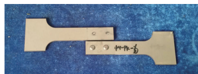
图5 普通铆接疲劳试验典型破坏模式—钉断 Fig.5 Typical failure mode of general riveting fatigue test—nail broken
