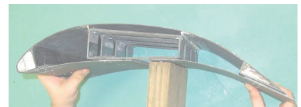
图5 “叠片式”蒙皮的应用 Fig.5 Application of semi-rigid skin
