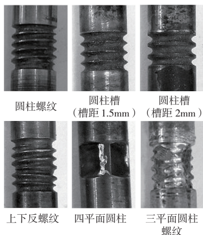
图2 不同特征的搅拌针 Fig.2 Probes with different characteristics
