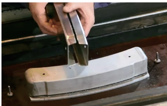
图2 相同材料用不同压力的回弹 Fig.2 Springback of the parts under different pressure with the same material
