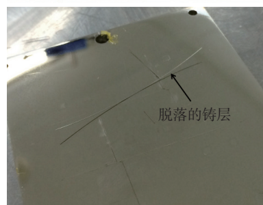
图9 铸层翘起及脱落 Fig.9 Tilting and abscission of cast layer
