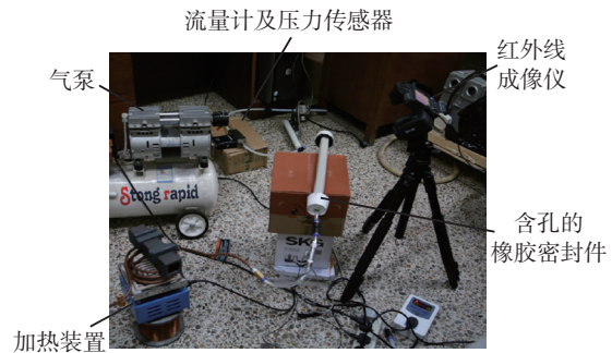
图6 红外测试技术试验装置 Fig.6 Experimental device diagram of infrared test technology
