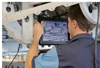
图4 应用MiRA/SART的A400M线缆装配 Fig.4 Application of MiRA/SART on A400M cable assembly site
