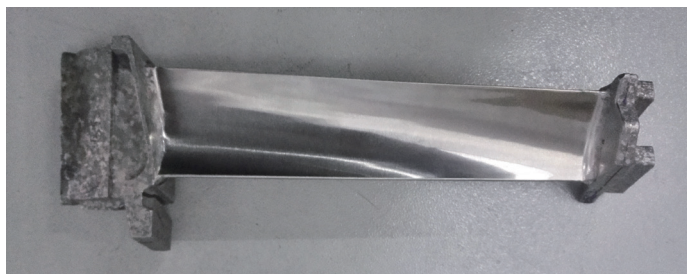
图6 镍基高温合金磨削后的表面 Fig.6 Surface after grinding nickel-base superalloy
