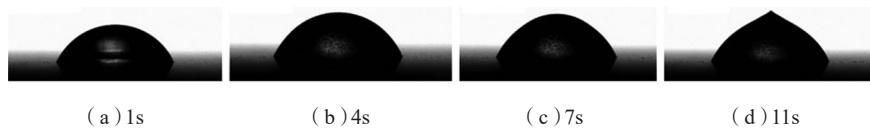
图6 -5°C条件下原金属表面结冰的过程 Fig.6 Freezing process of the original metal surface at -5 °C
