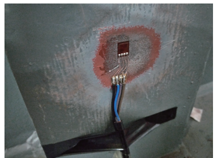
图8 载荷传感器布置 Fig.8 Load sensor arrangement
