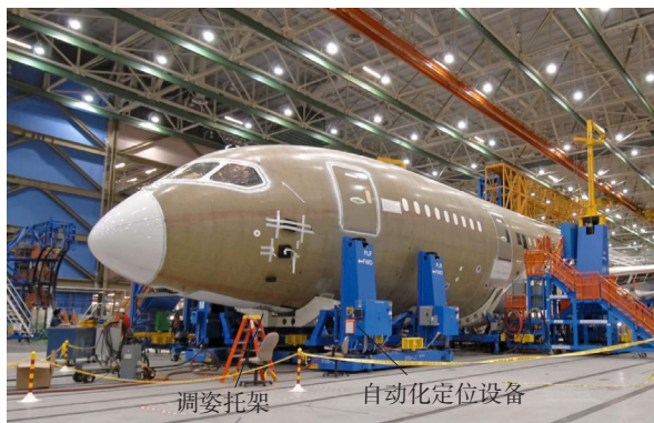
图8 采用托架式支撑装置的波音787机身自动化对接 Fig.8 Automatic docking of Boeing787 fuselage with bracket support
