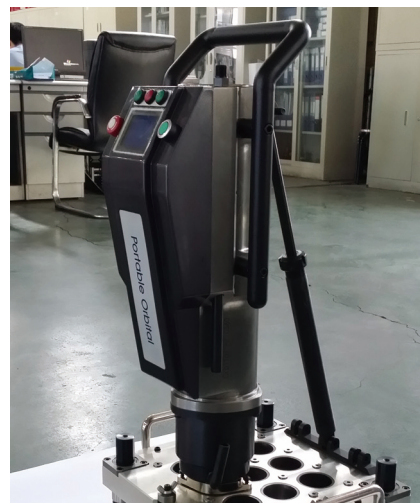
图9 便携式螺旋轨迹制孔装置验证机 Fig.9 Verification machine for portable spiral trajectory drilling device
