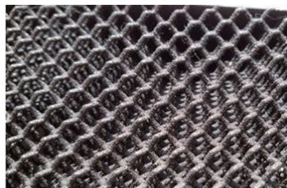
图 17 激光选区熔化制件原始表面 Fig.17 Original surface of laser selective laser melting part
