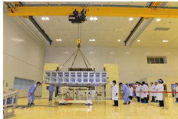
(e) 将长桁定位预组合模吊离气垫车
