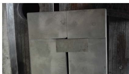
图16 长桁工装组合后台阶位置不匹配 Fig.16 Misalignment of step positions after string tooling assembly
