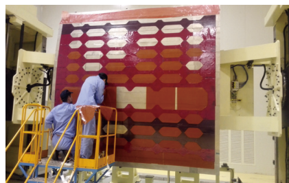
图11 填充硅橡胶垫 Fig.11 Silicone rubber pad laying up
