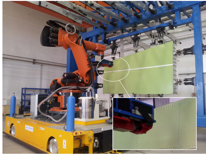
图11 翼盒模拟件机器人制孔系统 Fig.11 Verification of robot drilling system
