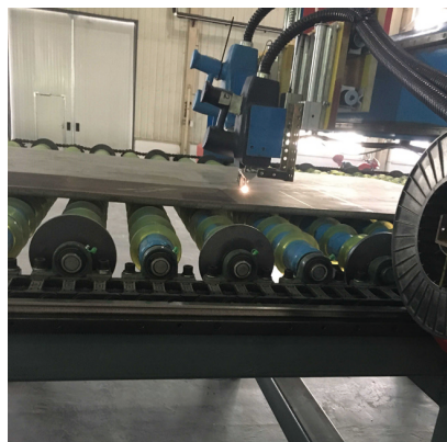
图11 自主研发激光器激光除漆过程 Fig.11 Process of laser painting removal by the independent-developed laser
