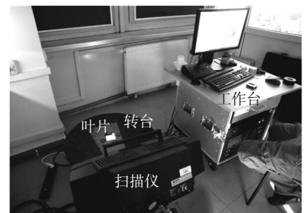
图12 ATOS II Triple Scan Blue Light 测量系统 Fig.12 ATOS II Triple Scan Blue Light measuring system
