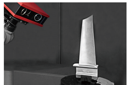
图11 Atos Core 结构光测量系统 Fig.11 Atos Core structured light measuring system
