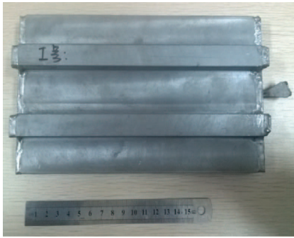
图31 热等静压后的预制坯 Fig.31 Preform after HIP
