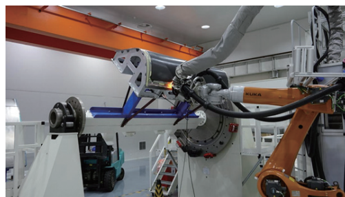
图9 吊挂前缘左侧段的铺放 Fig.9 Layup of left part of pylon upper fairing
