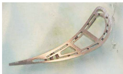
图 11 双层壁结构单晶叶片结构剖切示意图 Fig.11 Schematic of double-wall structure of single crystal blade
