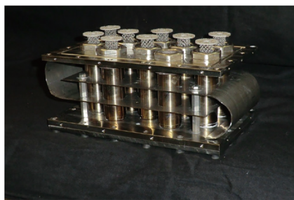
图12 具有10个反应管的氢释放装置 Fig.12 Hydrogen release unit consisting of ten parallel reactor tubes
