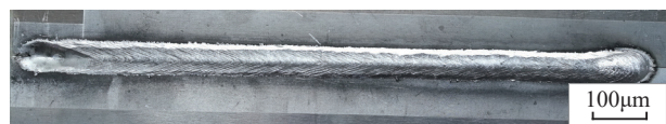
图 13 6mm厚铝合金锁底板焊缝外观 Fig.13 Weld appearance of 6mm thick aluminum alloy locked plate
