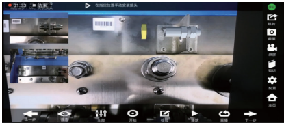
图8 零件机上装配操作智能引导 Fig.8 Intelligent pilot for part assembly operation
