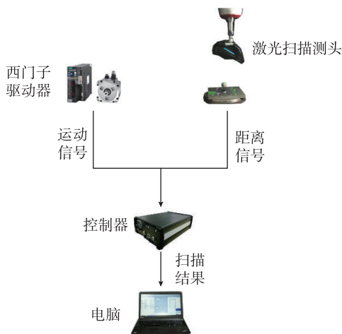
图5 线激光扫描硬件系统示意图 Fig.5 Schematic diagram of scanning system
