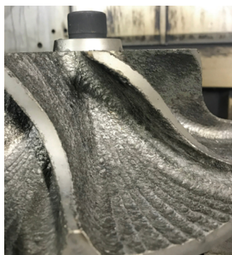
图7 中等能量电弧加工的流道 Fig.7 Channel machined in mid-energy
