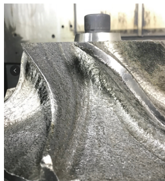
图8 小能量电弧加工的流道 Fig.8 Channel machined in small-energy
