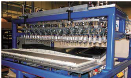
图7 CH-53K型机无轴承尾旋翼:自动铺层设备示意图 Fig.7 Bearingless tail rotor of CH-53K ATP equipment
