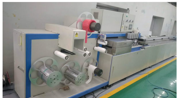
图7 填充芯材连续成型设备 Fig.7 Molding equipment for core filling material
