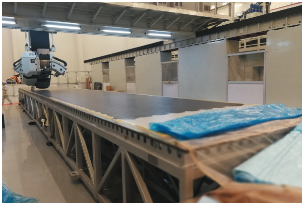
图4 铺带机铺叠预浸料平面毛坯 Fig.4 ATL machine preparing the flat blank
