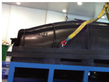
图15 改进前工装合模制造零件实物图 Fig.15 Parts made by mould-closing tooling before improvement
