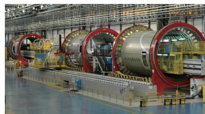
图2 波音787机身段自动钻铆系统 Fig.2 Automatic riveting system of Boeing 787 fuselage section
