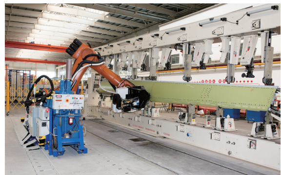
图10 外襟翼自动制孔试验 Fig.10 Automatic drilling experiment of out flap
