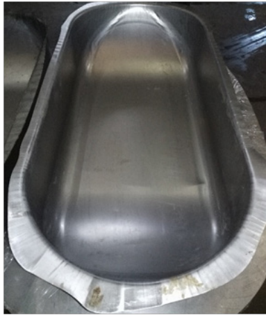
图10 充液拉深未切割整流罩零件 Fig.10 Part of hydroforming
