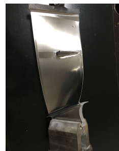
图6 机器人砂带磨削后的叶片表面 Fig.6 Blade surface after robotic abrasive belt grinding
