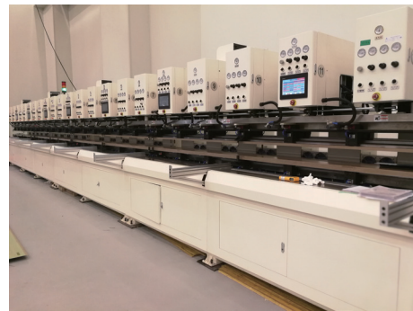
图8 专用叠层滑移成型设备 Fig.8 Laminated slip machine
