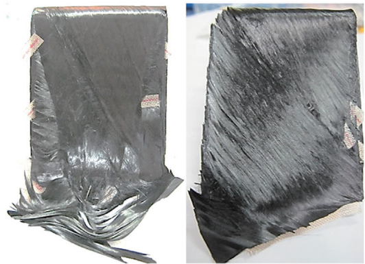
图22 纤维在平面内出现弯曲或开裂 Fig.22 Fiber bends and cracks in plane
