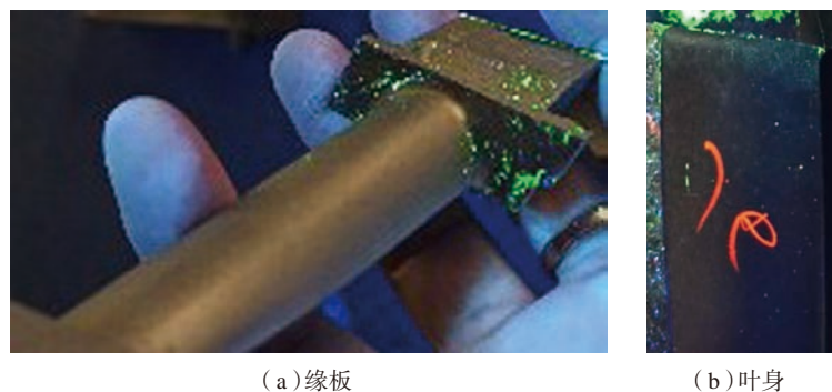
图2 叶片荧光显示部位及形貌 Fig.2 Leaf fluorescent display parts and morphology
