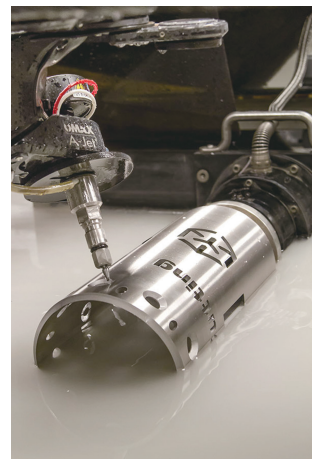
图2 五轴水切割机 Fig.2 Five-axis water jet cutting machine
