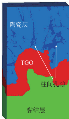
图8 EB-PVD热障涂层FIB-SEM三维成像 Fig.8 Three-dimensional imaging of EB-PVD thermal barrier coatings by FIB-SEM
