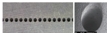
图 13 孔口形貌良好的气膜孔 Fig.13 Gas holes with good orifice morphology
