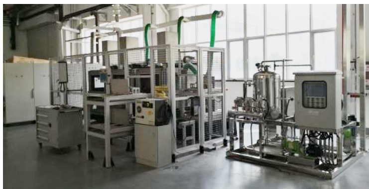
图7 多工位电液束加工设备 Fig.7 Multi-station equipment of electro stream machining
