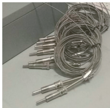
图5 压簧式K型热电偶 Fig.5 Pressure spring type K thermocouple
