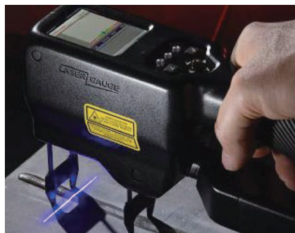
图 9 LaserGauges 激光测量系统 Fig.9 Laser measurement system of LaserGauges
