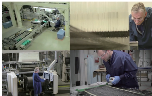
图 9 Leap-X 发动机风扇叶片三维机织过程 Fig.9 3D weaving process of Leap-X aero-engine fan blades
