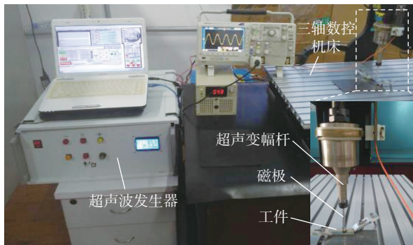
图 1 UAMAF 试验装置 Fig.1 Experimental setup of UAMAF
