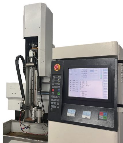
图 5 微小孔复合加工装备 Fig.5 Micro-hole composite processing equipment
