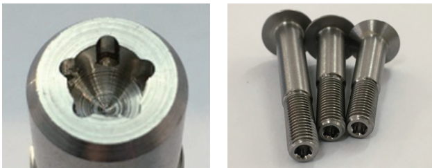
图 4 冲制的五瓣花形槽 Fig.4 Punched five-petal flower groove
