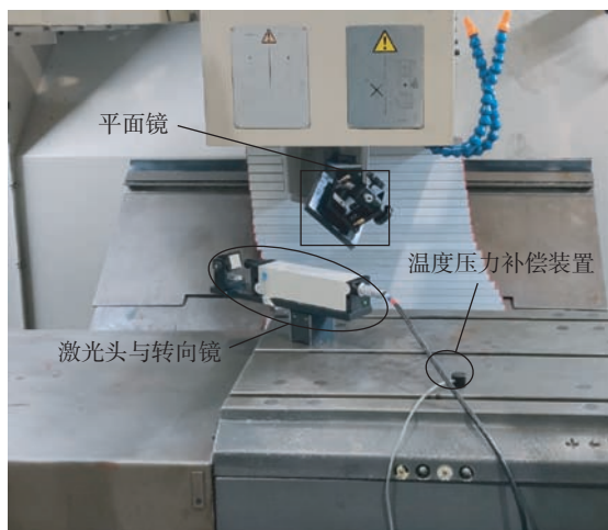
图 7 分步体对角线法误差测试 Fig.7 Method of sequential step diagonal error test
