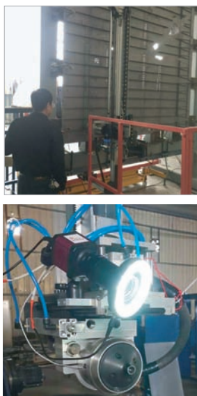
图13 国产半自动化电磁铆接系统 Fig.13 Domestic semi-automatic electromagnetic riveting system
