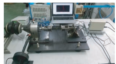
图 3 电磁加载中应变率动态拉伸测试装置 Fig.3 Medium strain rate dynamic tensile test device using electromagnetic loading
