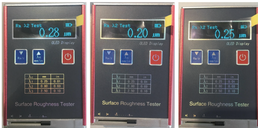
图 13 磨抛后叶尖表面粗糙度 Fig.13 Surface roughness of the leaf tip after grinding
