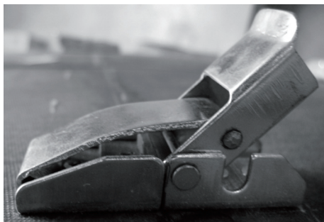
图5 天线主面分瓣连接件 III Fig.5 Connector III of antenna main surface sub-valve
