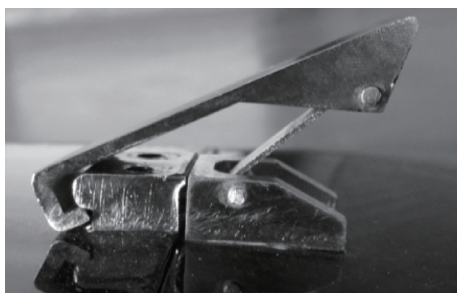
图4 天线主面分瓣连接件 II Fig.4 Connector II of antenna main surface sub-valve
