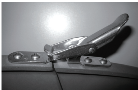
图3 天线主面分瓣连接件 I Fig.3 Connector I of antenna main surface sub-valve
