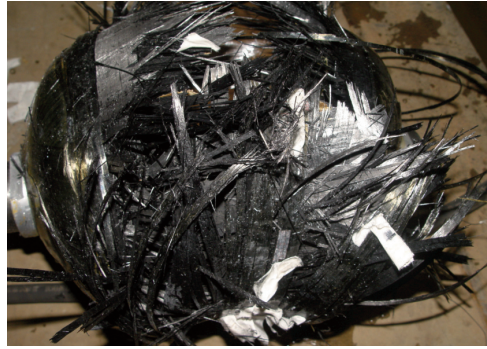
图5 爆破后的壳体 Fig.5 Case after water pressure burst
