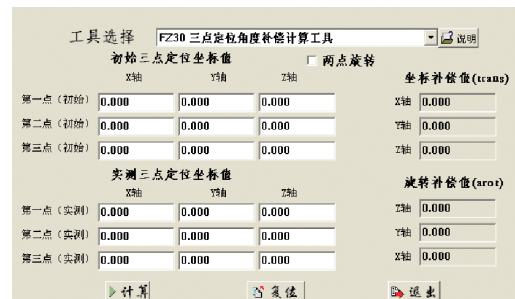
图6 软件实现空间旋转角度计算示例 Fig.6 Calculation of compensation angle for rotation in software
