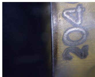
(c) 切削液冷却,切削 10min
